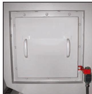
Side cleanout door with safety interlock
