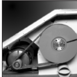
Dual solid flywheels offer heavy duty cutting inertia.
