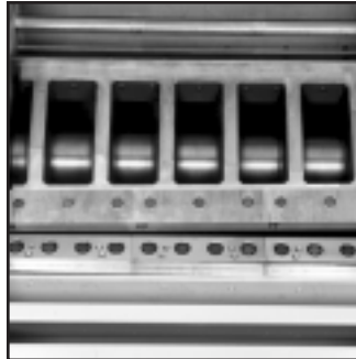
High carbon, high chrome D2 knives for maximum knife quality and consistency. Solid knife carriers provide extra support.
